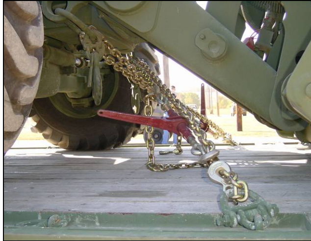
Figure 2-30. Front of BHL chassis properly tied down.
