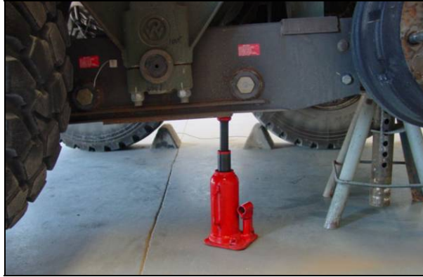
Figure 2-39. Proper Jack Location
