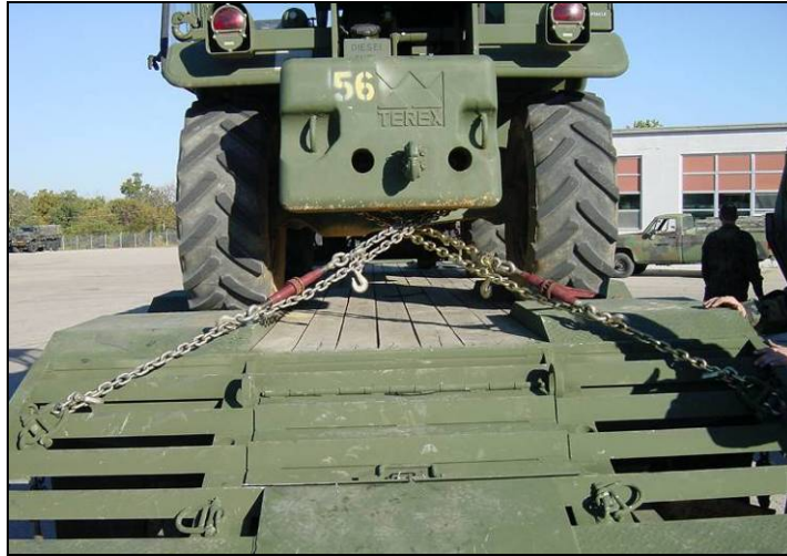
Figure 2-32. Rear of LRTF chassis properly tied.
