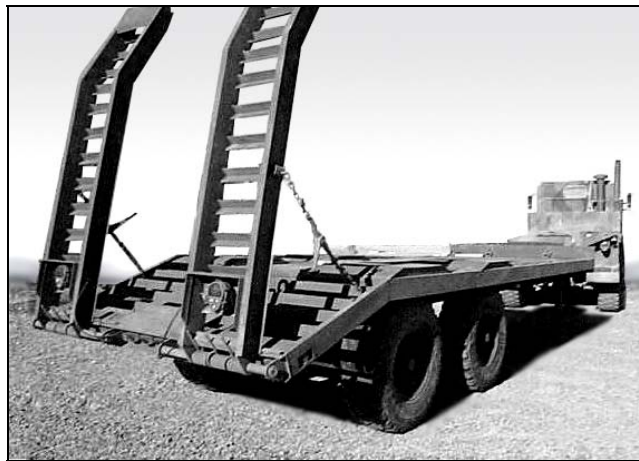
Figure 2-1. Loading Ramps in the Upright and Stowed Position
