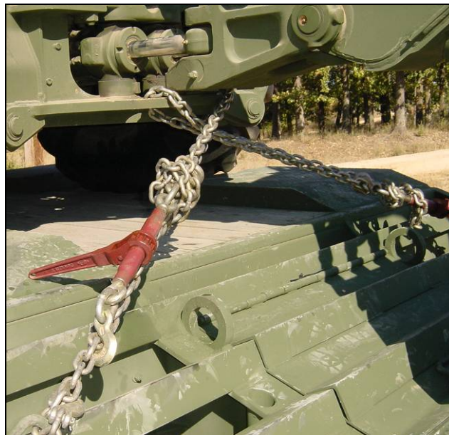
Figure 2-29. Rear of BHL chassis properly tied and tie down chains secured.
